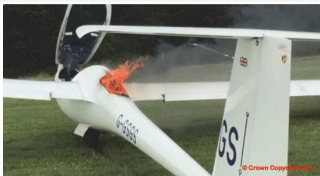
FIRE BLEW HATCH COVER OFF ON ROLLOUT. FLAMES WERE EXTINGUISHED BY FOAM-TYPE CHEMICAL
