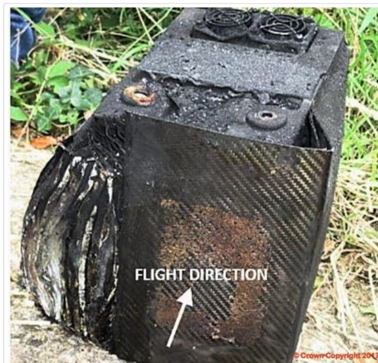
DAMAGE TO FRONT BATTERY BOX ON BRITISH SAILPLANE. BOTH INCIDENTS WERE "LUCKY" IN OCCURRING AFTER A SAFE LANDING
